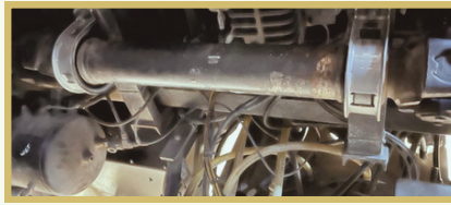
New carrier barrings for the pump drive line on E-721.
