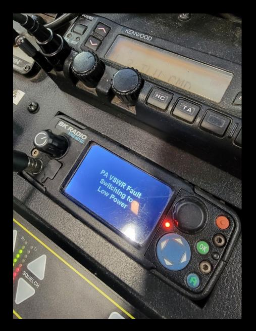
E-723 sustained damage to its radio antennas while responding to multiple incidents in the district. The antennas were taken out by a tree limb falling while the Engine was driving by.
