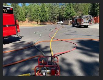
THFD staff pressure test all in-service fire hoses. All attack lines (1.5-2.5) will get pressurized to 300psi for 5 minutes, and all supply hoses (3 in - 5in) will get pressurized to 250 psi.
